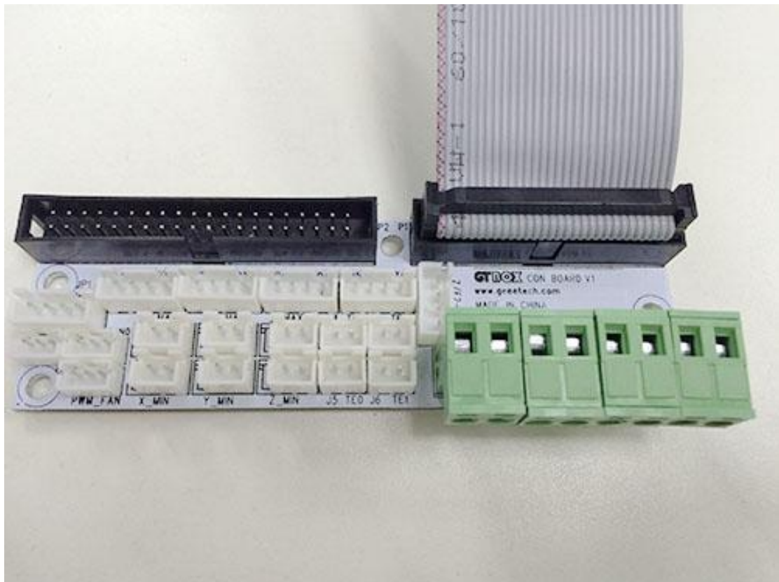
Step6. Connect the flat ribbon wire
