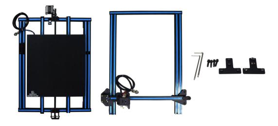
Step 2. Place the vertical frame parts on the bottom frame one (Note: Just keep the ends of the blue strips on the two frames meet each other.)
