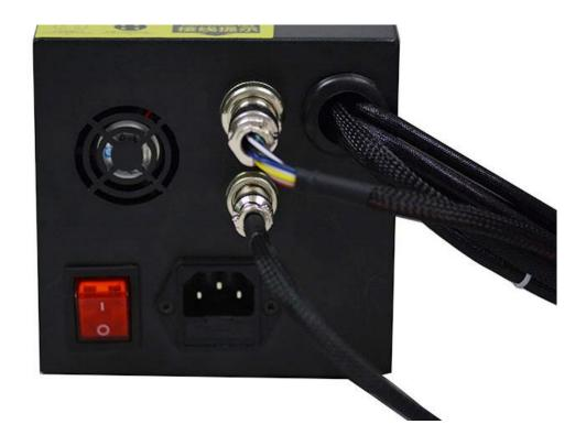
Step 6. Fasten the PTFE pipe (for loading filament).
