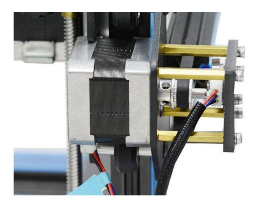
Step 2. Connect the two wires for the extruder and filament detector.
