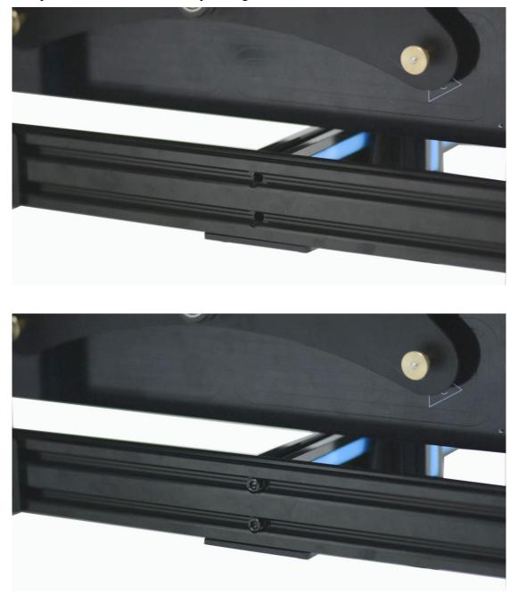
Step 5. Tighten the screws on the Z axis stators.
