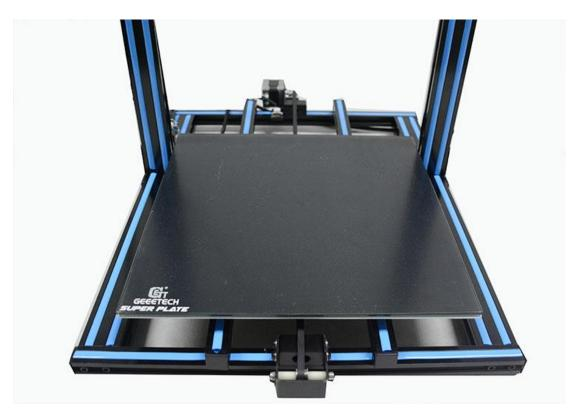
Step 3. Fix the two Z axis stators on two sides of the vertical frame respectively. Fasten the screws on the stators in a relatively loose way.
