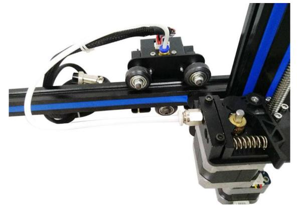
Though the other end of the PTFE pipe is pre-assembled, please make sure that it reaches the bottom of the printing head.
