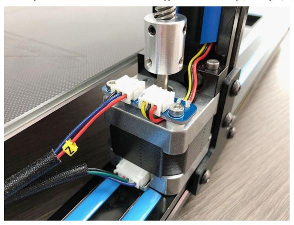
Step 4. Connect the two wires for Y axis stepper motor and endstop.
