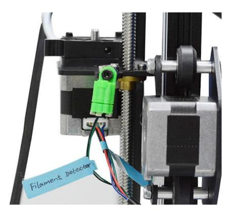
Step 3. Connect the two wires for Z axis stepper motor and endstop (the left port).
