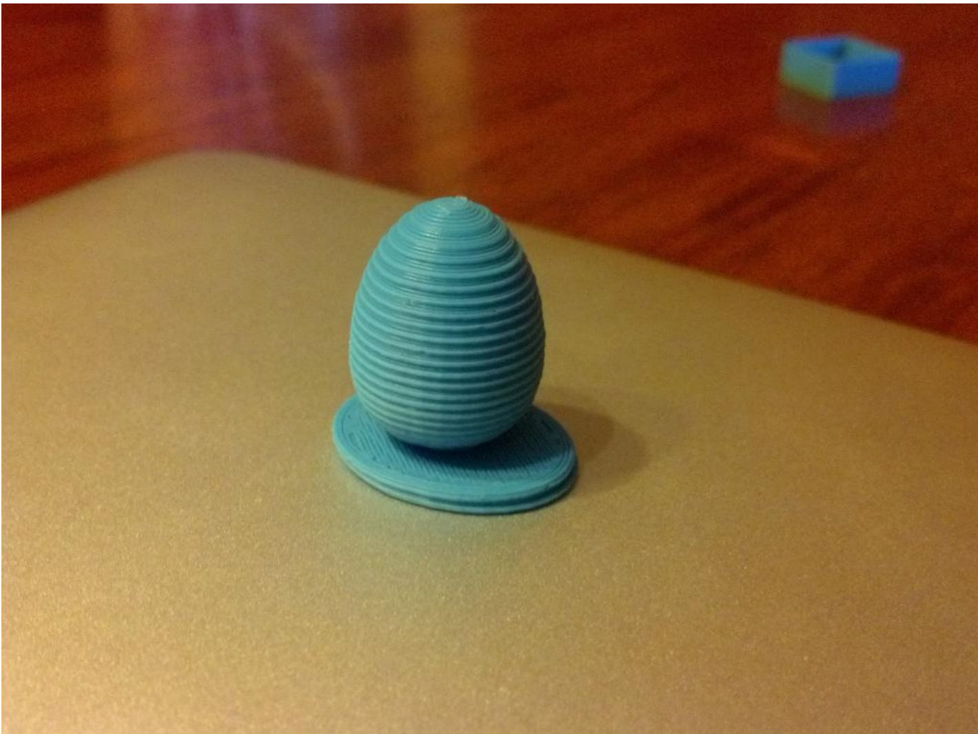
Z ribbing due to using non-metric screws. Photo credit: Jason Gullickson
