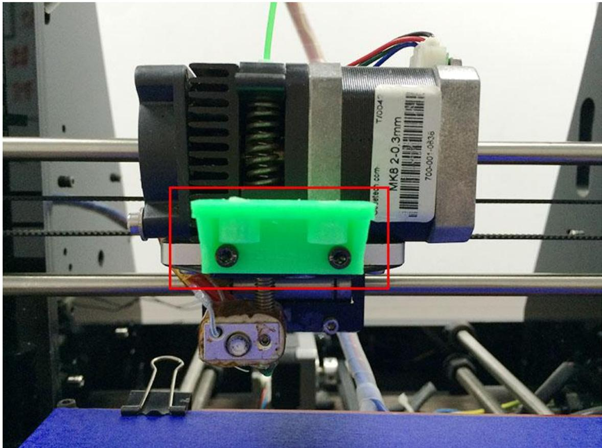
3. Fix the 3D Touch sensor on the sensor mount with 2 M3\*16mm screws and 2 M3 nuts.
